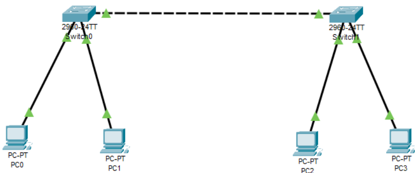
Gambar 10.2 Model Topologi Jaringan VLAN Mode Trunk
