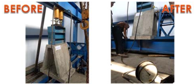
Figure 2. Model and testing Precast foundations
